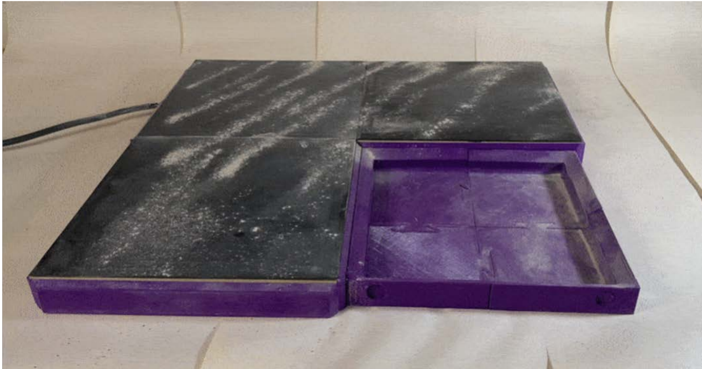
Three HOMES panels oriented 90 degrees with respect to the next and one collection panel
